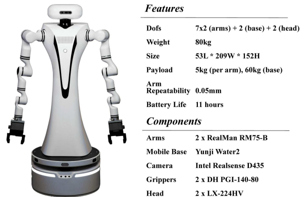
Fig. 5. Visual appearance and configurations of our bimanual mobile robot.
